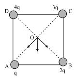
So, the net electric field will be along bisector of angle *AOB* which parallel to *CB*.
