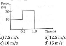
96. Force is applied to a body of mass 2kg at rest on a frictionless horizontal surface as shown in the force against time (F – t) graph. The speed of the body after 1 second is
