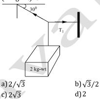
426.A body of weight 2 kg is suspended as shown in figure. The tension  $T_1$  in the horizontal string (in kg-wt) is
