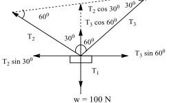
Now,  $T_2 \cos 30^\circ + T_3 \cos 60^\circ = T_1 = 100$
