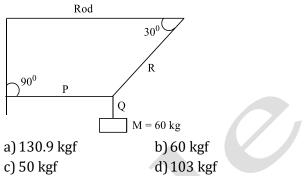
55. A body of mass 60 kg suspended by means of three strings P, Q and R as shown in the figure is in equilibrium. The tension in the string P is
