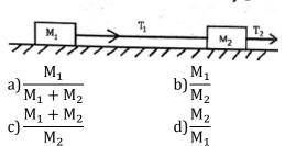
339. Two masses M<sub>1</sub> and M<sub>2</sub> are accelerated uniformly on frictionless surface as shown in figure. The ratio of the tensions  $T_1/T_2$  is
