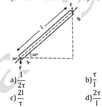
415. A rod 'l' m long is acted upon by a couple as shown in figure. The moment of couple is ' $\tau$ ' Nm. If the force at each end of the rod, the magnitude of each force is (sin 30<sup>0</sup> = cos 60<sup>0</sup> = 0.5)
