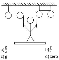
319.A man of mass m stands on a platform of equal mass m and pulls himself by two ropes passing over pulleys as shown in figure. If he pulls each rope with a force equal to half his weight, then his upward acceleration would be
