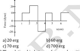
309. The relationship between force and position is shown in figure given (in the dimensional case). The work done by the force in displacing a body from x = 1 cm to x = 5 cm is
