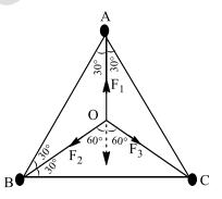
Resolving all the forces  $F_1$ ,  $F_2$  and  $F_3$  in vertical direction.
