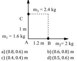
444. Three point masses  $m_1$ ,  $m_2$  and  $M_3$  are placed at the corners of a thin massless rectangular sheet (1.2 m × 1 m) as shown. Centre of mass will be located at the point?
