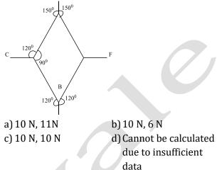
43. The below figure is the part of a horizontally stretched note. Section AB is stretched with a force of 10 N. The tension in the section BC and BF are
